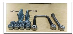
TORQUE SPEFCIFICATIONS for the ¼ - 20 nuts on the U-Bolt and 2" center bolt: 5 lbf-ft (24bf-in) (2.7 N-m). This is very slight pressure! Periodically check the tightness of all fasteners.
