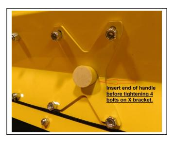
Step 4: Lock handle in place with 2" bolt and nut. The handle core is solid at this end. Even so, do not overtighten U bolt and the 2" bolt. Tighten the U bolt until a small crease forms in the braces as shown in the photo. Lastly, tighten the 2" bolt. Assembly is complete.
